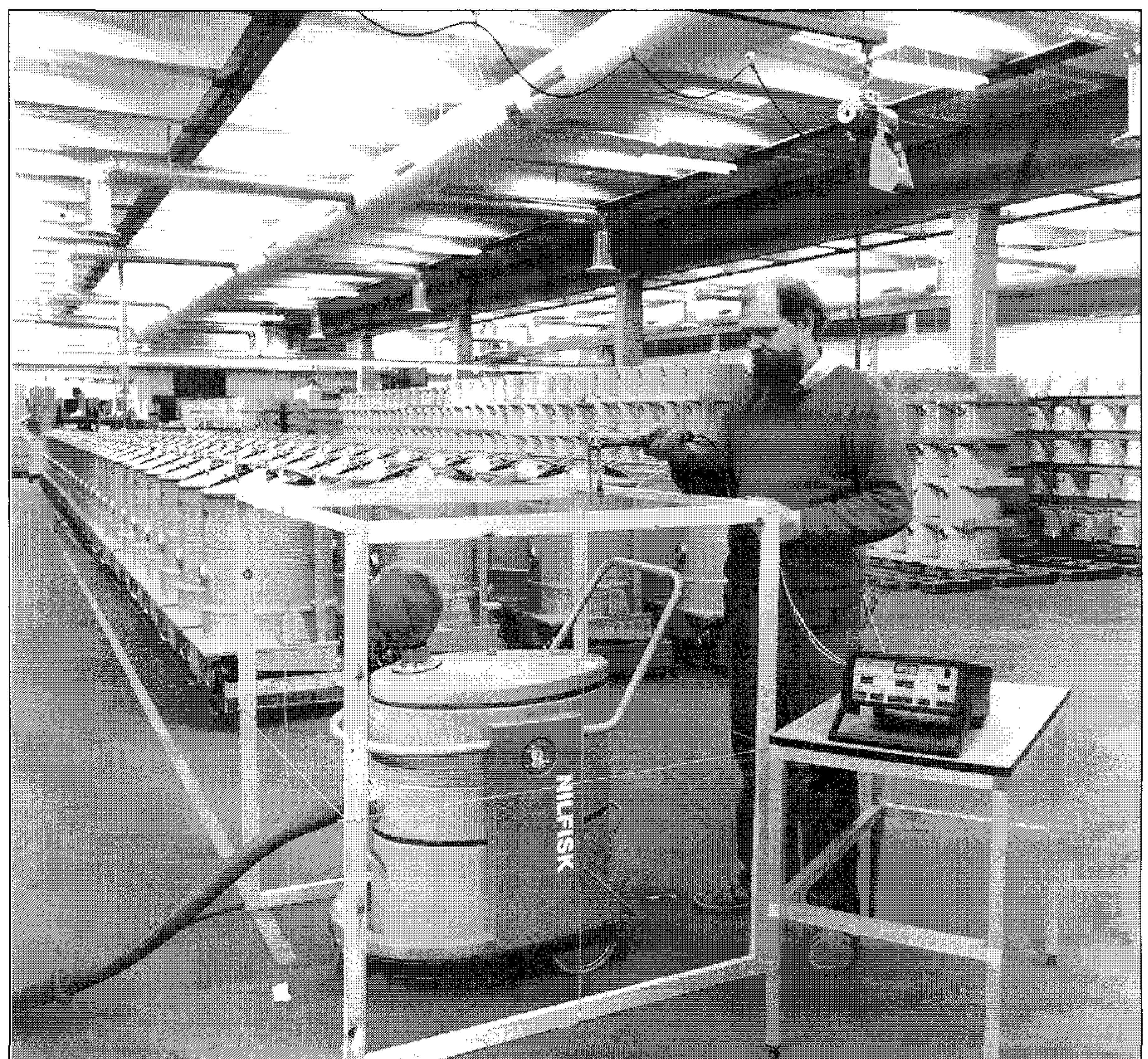
Fig.10 Set-up for sound power determination of a Nilfisk industrial vacuum cleaner (Courtesy of Fisker & Nielsen A/S)
